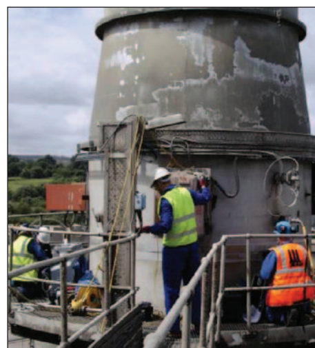
Figure 3: Sampling at the stack on the cement plant
