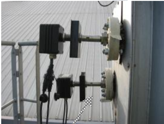
Water Build up on Upward Pointing Mounting
